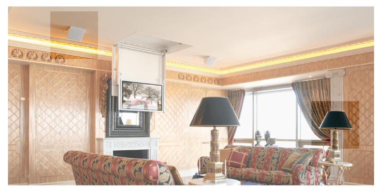
Sometimes custom installation needs something extra special and KEF's Ci200.2QT is just that. Easily configured for infrared remote control an integral DC motor allows you to position the speaker at the optimum angle with the press of a button. When fully retracted it can be operated as a conventional ceiling flush mounted speaker.
