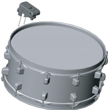
1. Use a drum key to loosen the RT-10S/RT-10T's sensor bolt.
