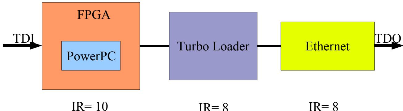
The Primary Image in the Flash ROM contains an embedded JTAG diagnostic port. This allows a user in Windows or Linux to debug software without an external JTAG cable. The internal JTAG diagnostic loopback looks just like a Parallel Port JTAG diagnostic cable when used with the Pico E-15 driver.
