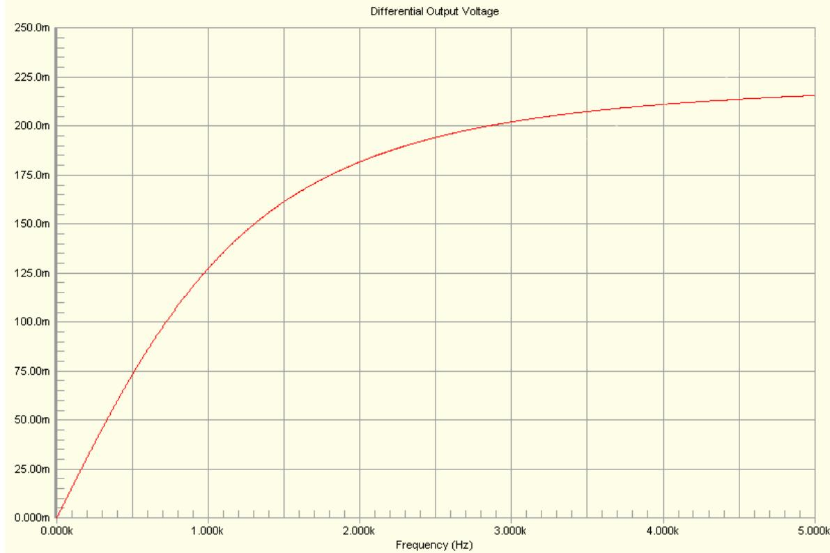
**DAC High Frequency Maximum Amplitude (50 Ohm Load)**
