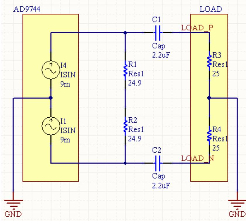
**DAC Low Frequency Maximum Amplitude (50 Ohm Load)**
