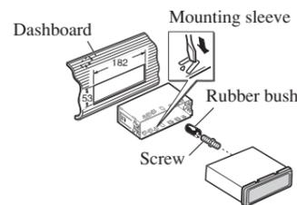
1. Insert the mounting sleeve into the dashboard.
