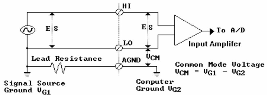
*Differential Configuration for Grounded Sources*
