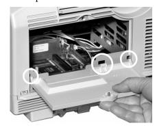
b. Swing the panel up and tighten the screw to secure it in place.
