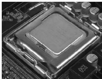
Align notches with notches on the CPU
