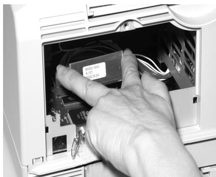
c. Press down on the card until it snaps into place and the gold contacts are fully inserted in the connector.
