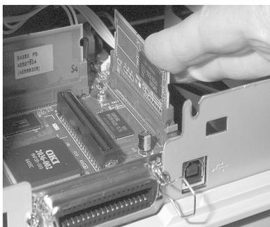
7. Check to make sure that both cards are fully inserted and installed correctly.
