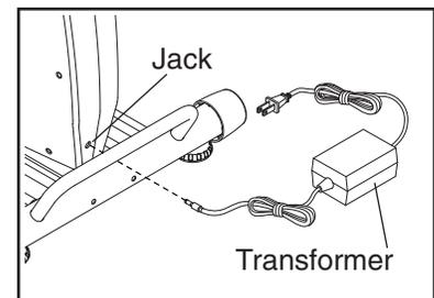
The motor may be heard while the elliptical trainer calibrates itself. **Important: Always plug in the transformer when using the elliptical trainer.** Note: When the power is on, the words MANUAL MODE will appear in the CROSSOVER TRAINING display. If the buttons are not pressed, the cables are not pulled, and the pedals are not moved for ten minutes, the console will go to sleep. Press any button to resume exercising.
