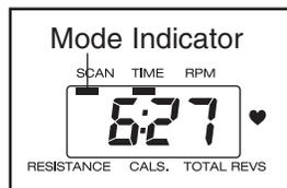
To select a single display mode, press the MODE button repeatedly until the desired mode indicator appears; make sure that the SCAN indicator does not appear. To reselect the SCAN display mode, press the MODE button until the SCAN indicator appears.
