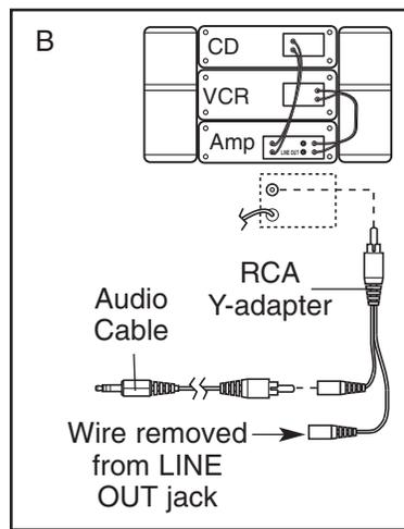
B. Plug one end of a 1/8" to 1/8" stereo audio cable (available at electronics stores) into the jack beneath the console. Plug the other end of the cable into a 1/8" Y-adapter (available at electronics stores). Plug the Y-adapter into the PHONES jack on your computer. Plug your headphones or speakers into the other side of the Y-adapter.
