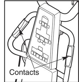
If your heart rate is not shown, make sure that your hands are positioned as described. Avoid moving your hands excessively or squeezing the metal contacts too tightly. For optimal performance, periodically clean the metal contacts using a soft cloth; **never use alcohol, abrasives, or chemicals.**
