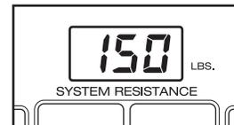
Next, press the SYSTEM RESISTANCE + and – buttons. Each time a button is pressed, the resistance setting will change by 1 pound. To change the resistance setting quickly, hold down one of the buttons.
