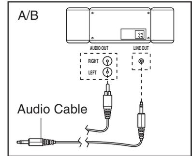
B. Refer to the drawing above. Plug one end of a 1/8" to 1/8" stereo audio cable (available at electronics stores) into the console iFIT jack. Plug the other end of the cable into the LINE OUT jack on your stereo.
