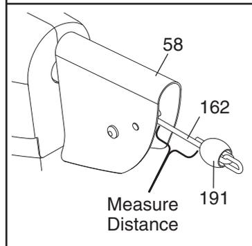
Set the elliptical trainer resistance to the lowest level. Have a second person pull the Rope (162) out and hold it while the Rope is adjusted. Push the Rope Cover (191) down the Rope and loosen the two M5 x 21mm Flat Head Screws (195). Pull the Rope through the Link (192) and the Rope Clamps (193, 194) to shorten the Rope by the measured amount. Then, retighten the two Screws and cover the Rope Clamps with the Rope Cover.
