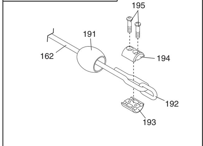
**WARNING:** Always make sure the two M5 x 21mm Flat Head Screws (195) are fully tightened before the elliptical trainer is used.
