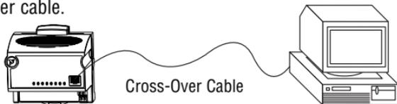
Do not use a cable longer than 100 m. If you are using a 100 Mbps Ethernet, National Instruments recommends using a Category 5 shielded twisted-pair Ethernet. If you need to build your own cable, refer to the FP-1600 User Manual for cabling details.
