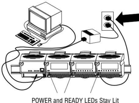
The **READY** LEDs will not light until an IP address is assigned. Likewise, the **STATUS** LED will stay lit until an IP address is assigned.
