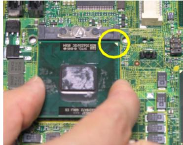
4. On the front end of the CPU socket is a locking mechanism designed into the form of a screw head. Make sure that you actuate or deactivate this mechanism with a screwdriver before and after installing the CPU.
