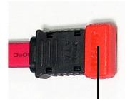
Take out the dust cover and connect to the hard disk devices
