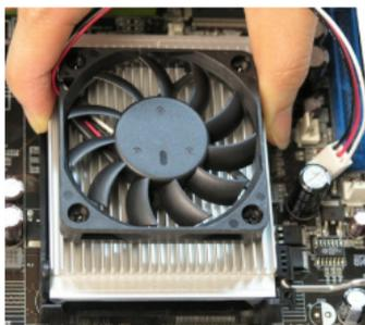
5. Mount the cooler set (fan & heatsink bundled) on top of the CPU and fit it into the retention mechanism.
