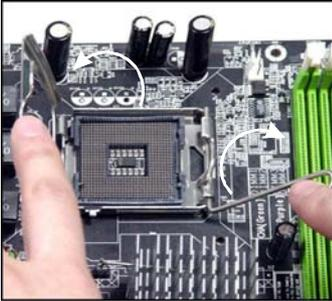
6. After confirming the CPU direction for correct mating, put down the CPU in the socket housing frame. Be sure to grasp on the edge of the CPU base. Note that the alignment keys are matched.
