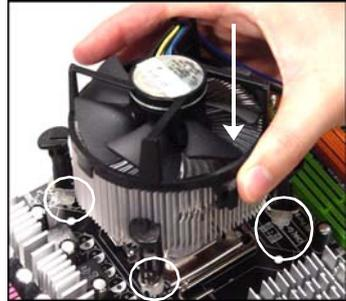
11. Press the four hooks down to fasten the cooler. Then rotate the locking switch (refer to the correct direction marked on it) to lock the hooks.
