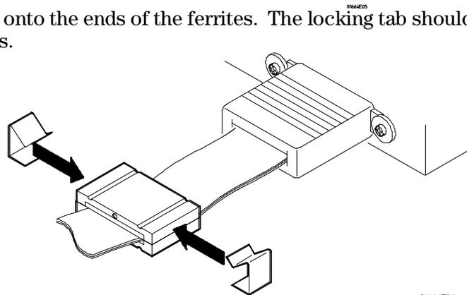
When properly installed, the ferrite should appear on the logic analyzer cable as shown.
