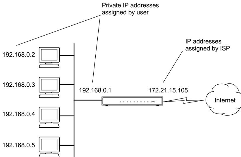
**Figure C-3: Single IP Address Operation Using NAT**
