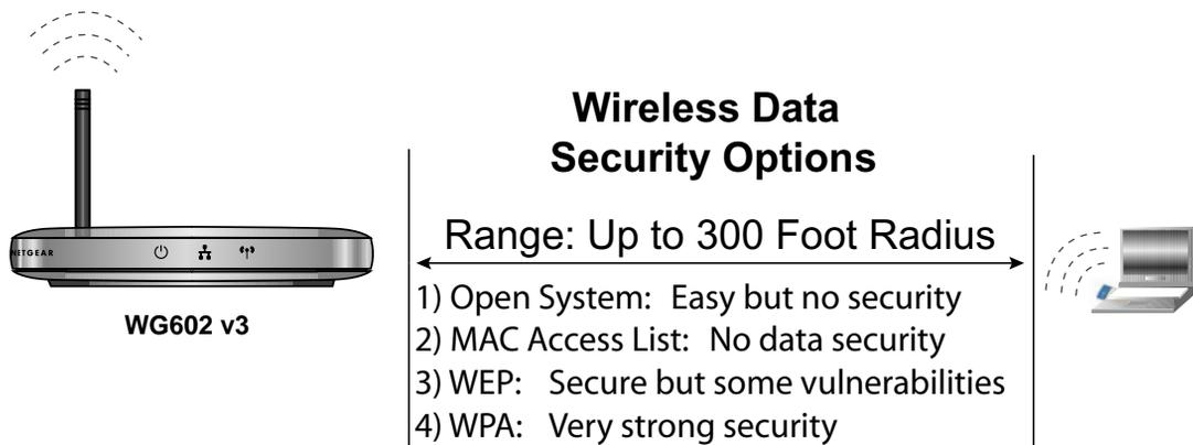
**Figure 3-1: WG602 v3 wireless data security options**
