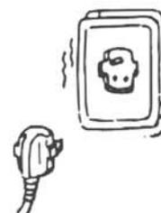
Make sure that the back of the unit is at least 5 inches or more away from a wall. To ensure proper air intake, do not place the unit in front of curtains or drapes. Route the power cord carefully to avoid a tripping hazard.
