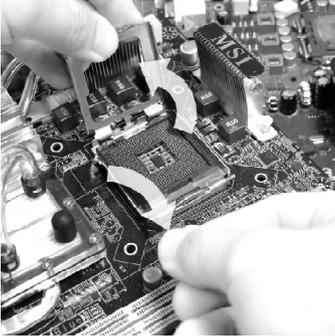
6. After confirming the CPU direction for correct mating, put down the CPU in the socket housing frame. Be sure to grasp on the edge of the CPU base. Note that the alignment keys are matched.
