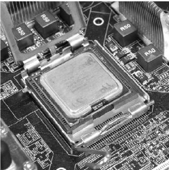
8. Cover the load plate onto the package.
