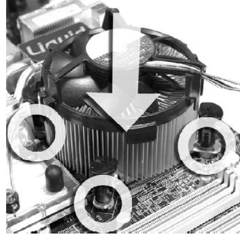
11. Press the four hooks down to fasten the cooler. Then rotate the locking switch (refer to the correct direction marked on it) to lock the hooks.
