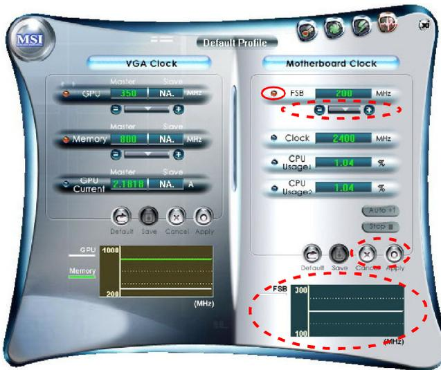
On the underside, it shows the graphs of the clocks. Only the curves of the item which the button is lit up with red color will be shown.
