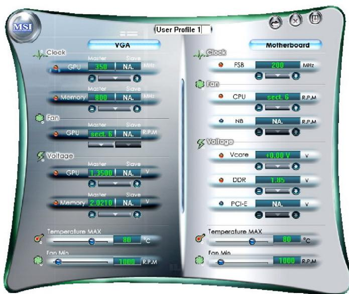
Use the draw bar to set the max system temperature. When the system temperature exceeds the threshold you defined, the system will pop up a warning message and shut down the system.
