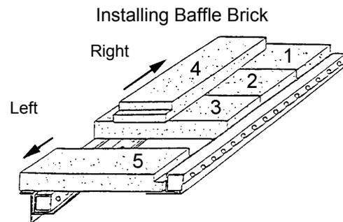
Top View of Baffle Brick Installed
