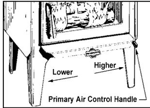
You will generally want to set the control in the low or medium range. The stove is safe burning on any setting as long as combustibles are kept at the specified safe distances.
