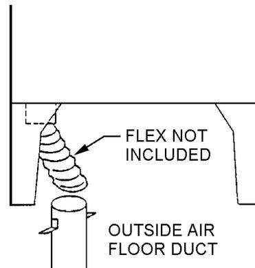
This appliance utilizes a 3" (76 mm) diameter outside air floor duct (Catalog # 14M66). Outside air can be taken from beneath the home or through an outside wall. The collar for connecting flex to stove in on the underside of the stove as shown here.
