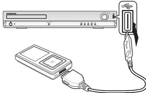
2 Press the **FUNCTION** button on the DVD Player or the **USB** button on the remote control to select the USB mode.
