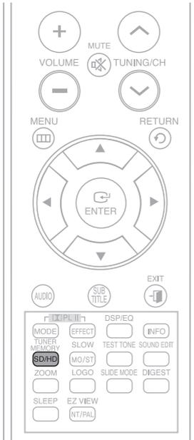
In Stop mode, press and hold the **SD/HD** (Standard Definition/High Definition) button on the remote control.
