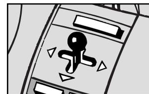
After the loop is completed, return TOGGLE to NEUTRAL position to level off.
