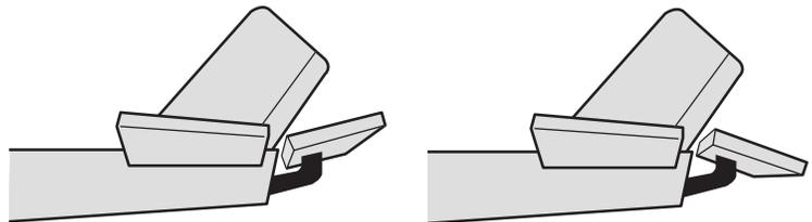
IF THE FLYING HEIGHT IS TOO LOW OR THE PLANE DOES NOT CLIMB, THE STUNT FLAP MAY NOT BE HORIZONTAL. ADJUST THE STUNT FLAP UPWARD UNTIL IT IS LEVEL WITH THE HORIZONTAL TAIL WING.
