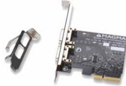
For low profile case applications, you may need to change the mounting bracket to the low profile bracket that shipped with your system. This is done by removing the screws that hold the card to the bracket. Be sure you are using proper ESD procedures when completing this action.
