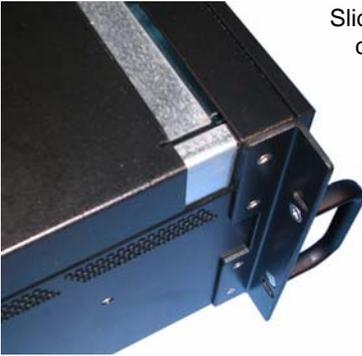
Slide the enclosure cover backward to disengage it from the guides at the front of the enclosure by firmly grasping the edges of the cover lip and pulling the cover backward about 1" until it clears the front hold-down, and then lift the cover off.
