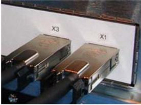
Connect cables to the chassis.
