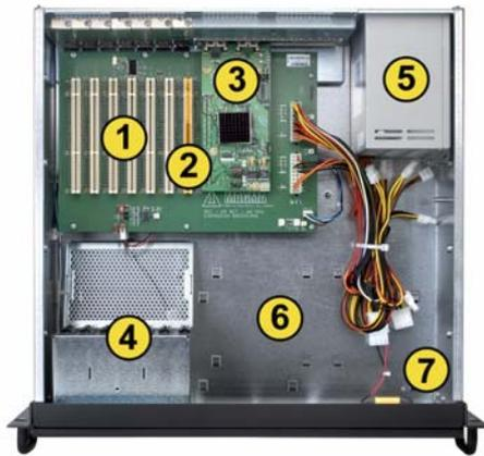
Be sure to keep the can of compressed air about six inches from the parts being sprayed with air. Pay particular attention to the fans in the chassis **4** and power supply **5** because they are critical to air movement to keeping your chassis cool. Also spray the PCI-X slots **1**, the backplane **3**, and the chassis bay areas **6** and **7**. If you have mounted hard drive cages in one or both of these areas, be sure to check for dust that can collect in the space between the drives.
