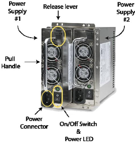
The redundant power supply includes two hot-swappable modules that share the power load requirements during normal operations. Should one module fail for any reason, the power load will be shifted to the other module and sound an audible alarm.
