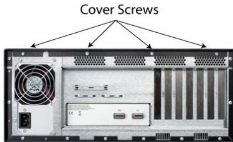
Remove all of these screws to open the enclosure.
