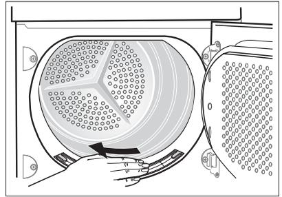
3. After a period of time, a patina due to detergent residue on laundry forms on the filters. When this occurs, clean the filters with warm water using a brush. Remove the filter from the door pulling it out. It can be positioned with the tooth facing to the left or to the right).
