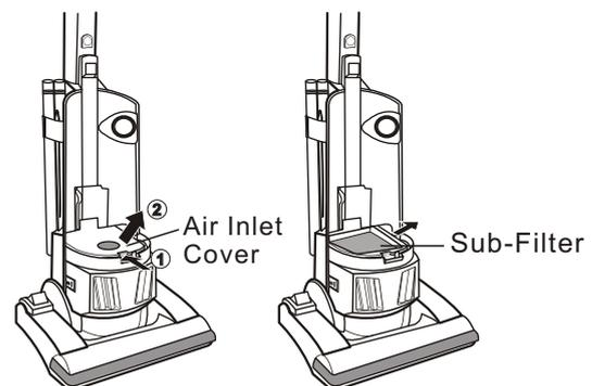
**Caution:** Do not wash the sub-filter in a washing machine, and do not use any other equipment such as a hair dryer to dry it. Always allow 24 hours for drying. Do not operate the vacuum without the sub-filter. Be sure the sub-filter is dry and properly installed. Failure to do so could result in electrical shock, personal injury, or motor failure.
