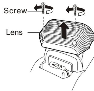
**3** When removing the headlight lamp, be careful not to pull on the headlight lamp wiring.
