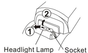
**5** Push a new lamp gently into the socket and turn it clockwise to tighten it.
