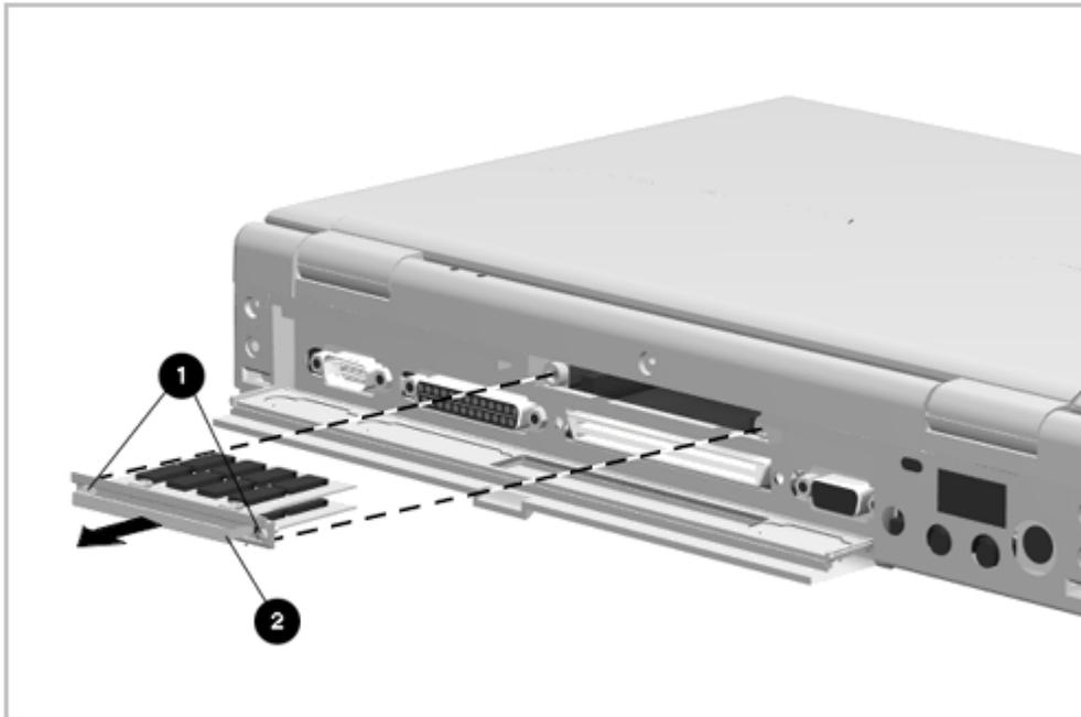
Figure 5-18. Removing a Memory Module
