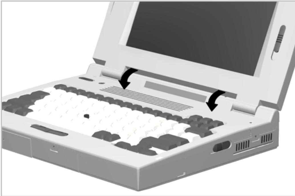
Figure 5-23. Removing the CPU Cover
