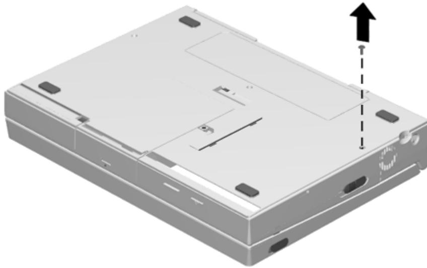
Figure 5-12. Removing the MultiBay Security Screw
