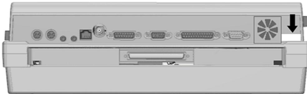
Figure 7-1. MultiBay-ISA Expansion Base Serial Number Location
