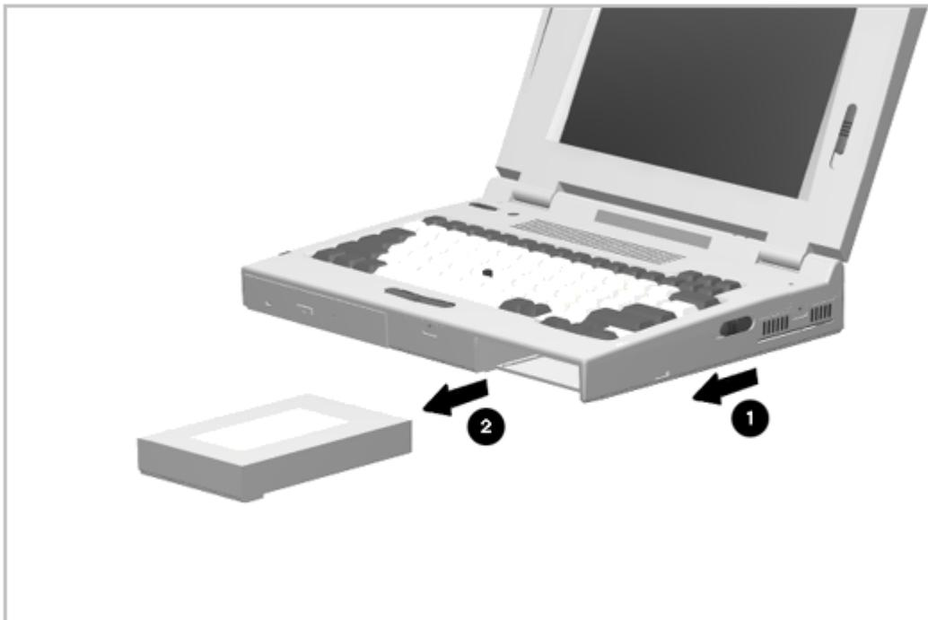
Figure 5-5. Removing the Battery Pack
