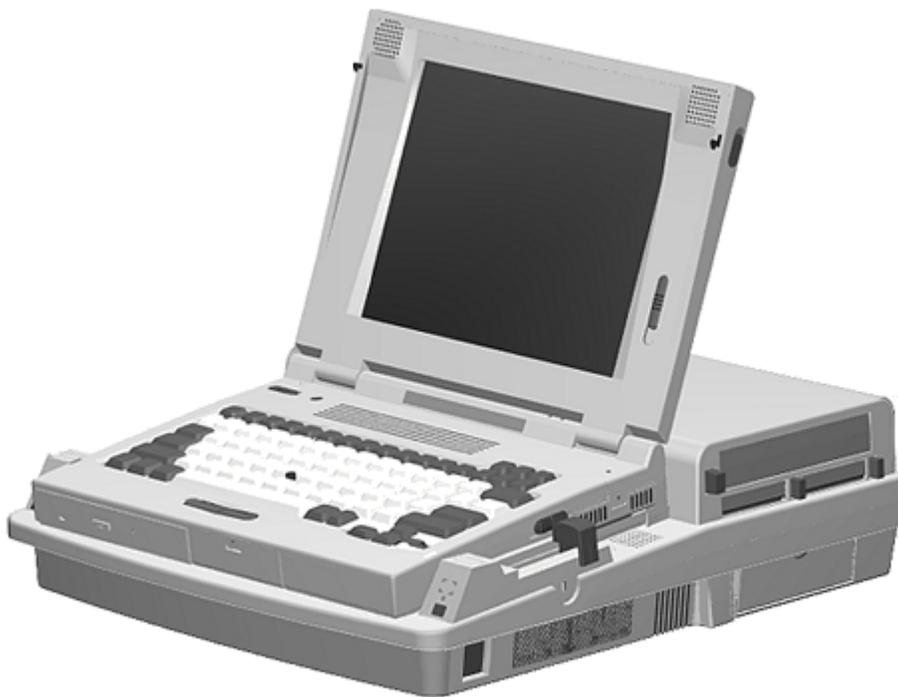
Figure 1-1. Compaq LTE 5000 Personal Computer with Optional MultiBay-ISA Expansion Base
