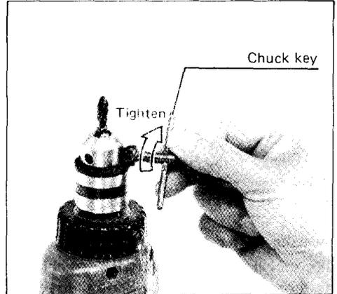
After use, return the chuck key to the storage cavity on the tool.
