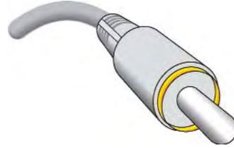
**Component: Y, Pb, Pr**—Use these cables to connect your component equipment. This connection provides the best picture, but does not include sound. (Cable colors: Y = green, Pb = blue, and Pr = red.)
