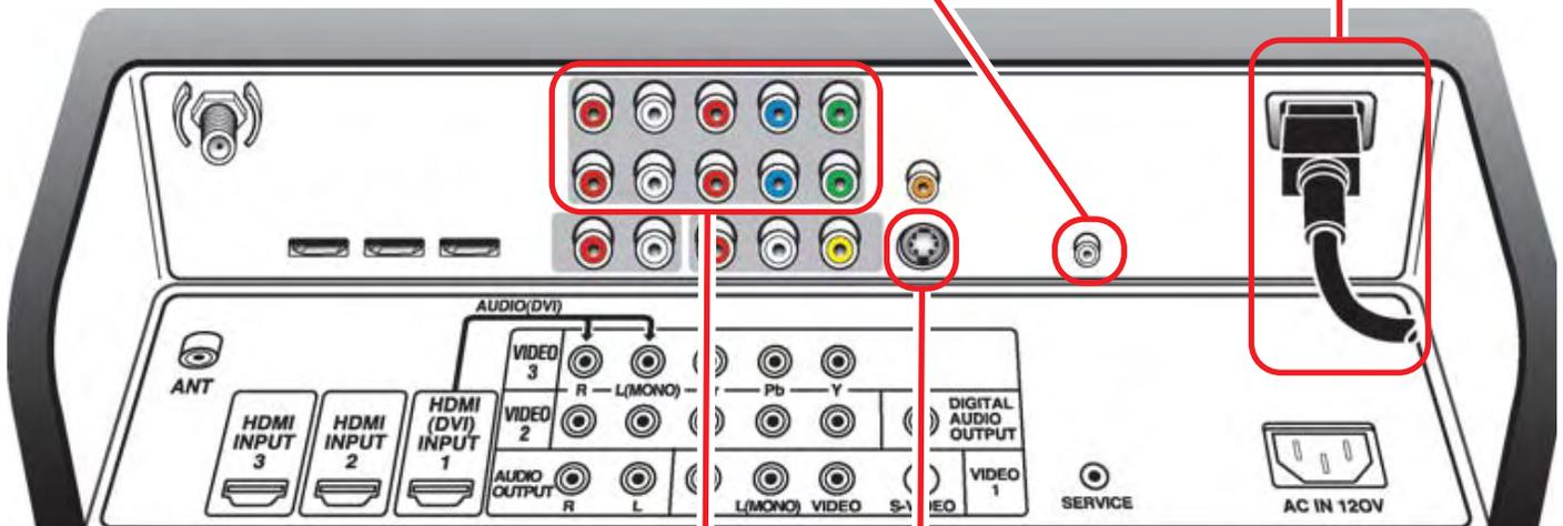
**Component Video Input (VIDEO2 or VIDEO3)**—Connect digital video equipment to the Y (green), Pb (blue), Pr (red) and Audio L/R jacks. These jacks will automatically detect the type of signal being received. **See PAGES 20, 21, and 22 for Component jack connections.**
