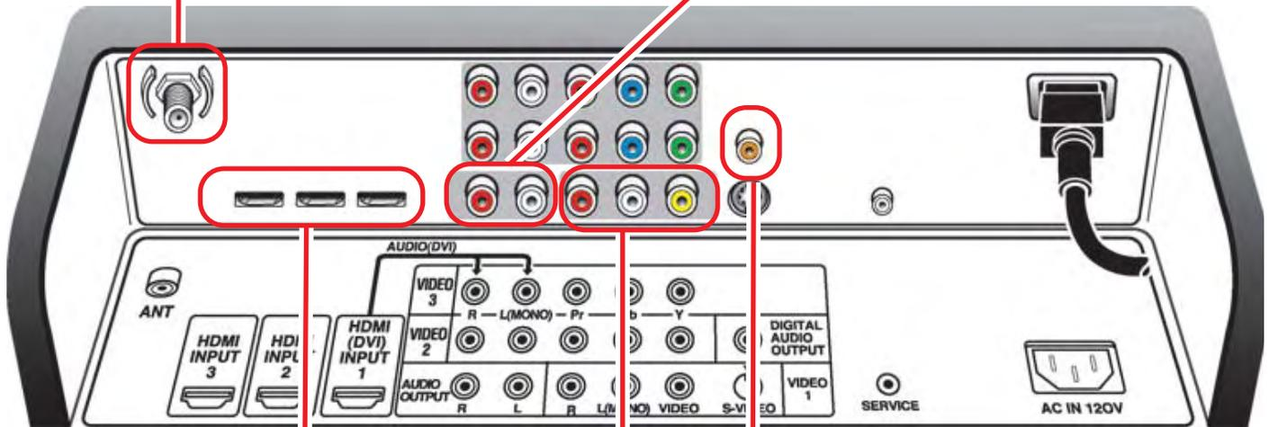
**HDMI INPUT1/2/3 (High-Definition Multi-media Interface), PAGE 7**—Connect digital video equipment to this jack. It takes only one cable (not supplied) to communicate between audio/video equipment and this DTV. HDMI (DVI) INPUT1 jack is compatible with DVI equipped AV devices. (Separate audio connection and an adapter are required for DVI device.) **See PAGES 18 and 19 for HDMI connection.**
