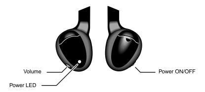
To turn the headphones on and off, push the Power ON/OFF button on the right ear piece. The Power LED on the left ear piece indicates when headphone power is on. Power shuts off automatically after 3 minutes of no audio to preserve battery life.
