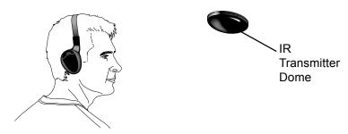
Using the headphones with your system allows rear-seat passengers to listen to their VCR or video game without disturbing front-seat passengers. When using the headphones the IR transmitter dome must have a direct line of sight to the headphones to work properly.
