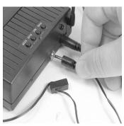
Plug the IR emitter cable into the back of the VCŘ Commander.
