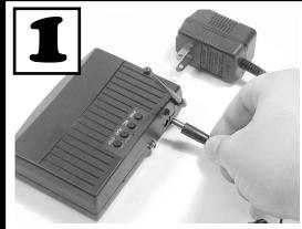
Connect the power supply to the VCR Commander and plug it into a wall outlet.
