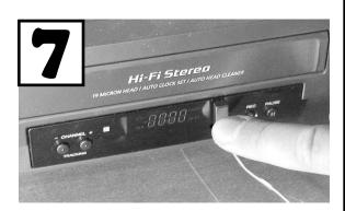
Press the emitter onto the VCR you are going to control, after removing the plastic from the adhesive backing.
