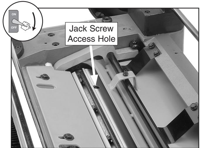
Figure 4. Jack screw access hole in the cutterhead.
