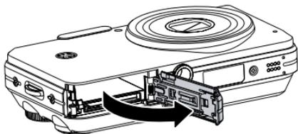
2. Insert the battery while observing the correct polarity. Use the side of battery to press down the stopper as shown, allowing the battery to be inserted properly.
