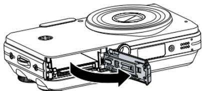
2. Insert an optional SD/SDHC card into the memory card slot as shown.
