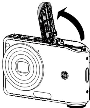
2. Insert the battery while observing the correct polarity. Use the side of battery to press down the stopper as shown, allowing the battery to be inserted properly.
