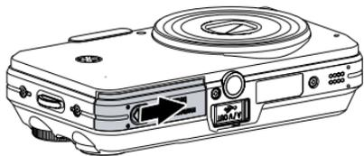
To remove the SD/SDHC card, open the battery compartment and gently push the card to release it. Pull the card carefully.
