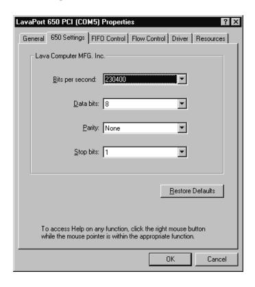
The data rate of the LavaPort may be set using the Bits per Second pull down menu.
