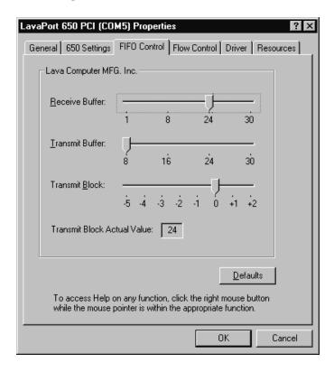
The LavaPort-650 uses a 16650 UART incorporating a 32-byte FIFO (first-in first-out) buffer.
