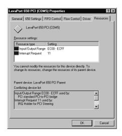
Because the LavaPort 650 is a PCI device, Windows will always allocate non-standard I/O resources to this port (e.g. Assigning it as Com 5, even though any one of Com1-4 may be free). If your software requires the use of standard I/O resources, you may modify those used by the LavaPort-650 in one of two ways:
