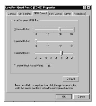
Each of the LavaPort-Quad's four ports incorporates a 64-byte FIFO (first-in-first-out) buffer.
