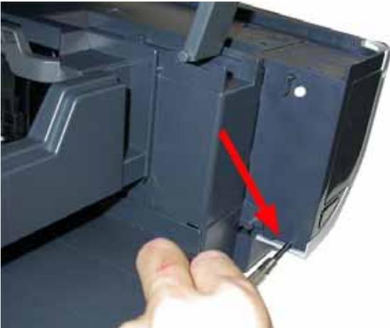
ii) Slide the side cover R2 toward the machine front, and remove it.
