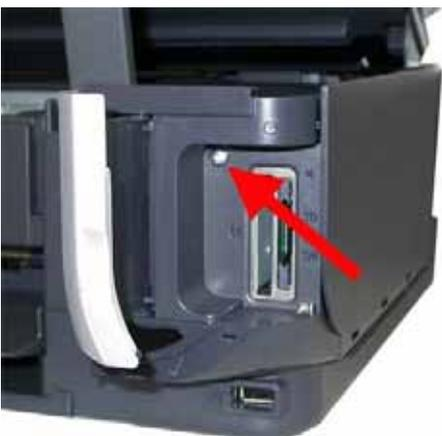
iv) Remove 2 hooks (No. 1 in the photo below). While pressing the lock pin (No. 2 in the photo below), slide the front cover R toward the machine front, and remove it.
