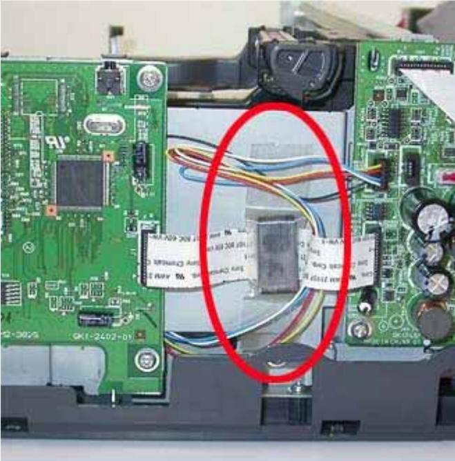
**(7) Carriage unit flexible cable wiring**
