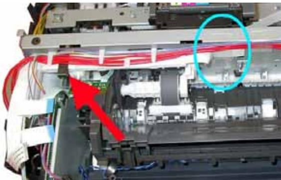
**(8) Power supply unit cable wiring**
