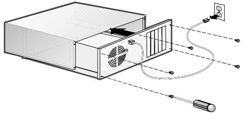
**4** Locate an unused PCI expansion slot (typically white or ivory) and remove the expansion slot cover. Save the slot cover screw for use in Step 6.
