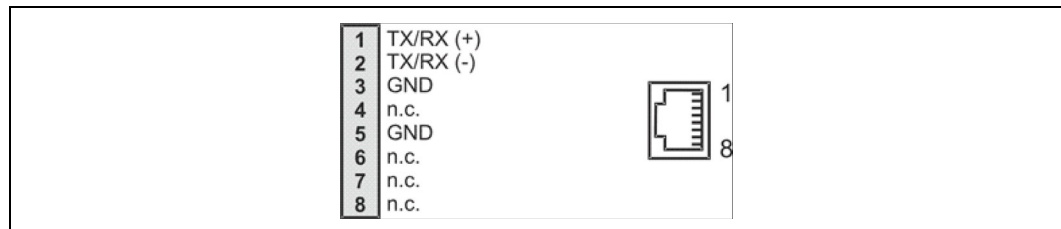
Figure 17. ICMB Connector Pinout
