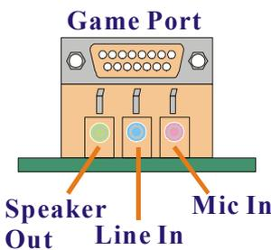
1. **Speaker Out** is used to connect to speakers or headphones. If the Super 5.1 driver is installed the Speaker Out becomes the Front Speaker.
