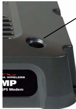
Figure 4-2: The MP modem reset button.
