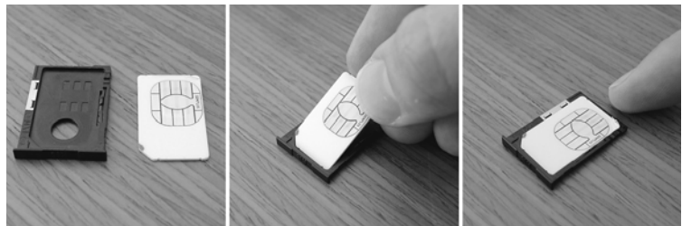
Figure 3-10: Placing a SIM card into the sled.
