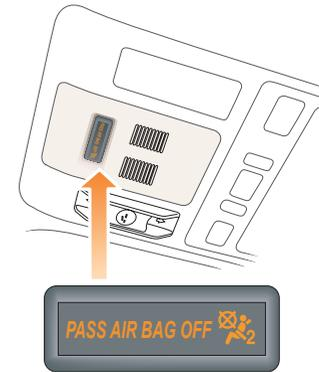
The front passenger seat is fitted with an occupancy sensor system that determines the state of seat occupancy and sets the status to suit:
