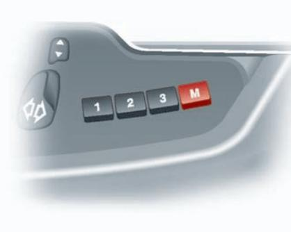
If button **1**, **2** or **3** is not pressed within seven seconds of the **M** button being pressed, the memory function will cancel.
