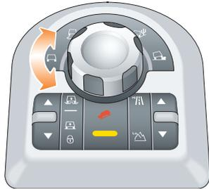
The Terrain Response system, if fitted, is always active and cannot be switched off. When the vehicle is started the system will normally start in its **General** program.
