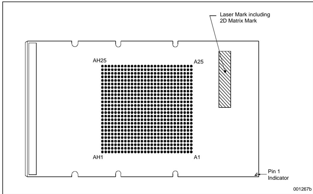
**NOTE:** 2D Matrix Mark only present on Itanium 2 processor (6 MB), Itanium 2 processor (4 MB) and Itanium 2 processor (1.3 GHz, 3 MB).
