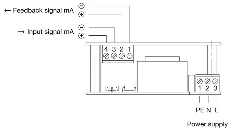
Wiring diagram for stroke length adjuster
