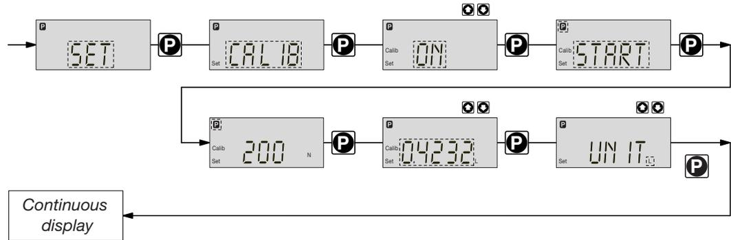
The S2Ca can also run in calibration mode. The corresponding continuous displays show the current dosing quantities or the feed rate.
