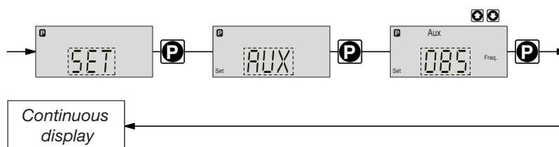
The programmable function “auxiliary frequency” allows switching to a different stroke frequency, which can be set in the AUX menu. It can be activated via the “external control” terminal. When the auxiliary frequency is activated, “aux” appears in the LCD display. This auxiliary frequency overrides the current stroke frequency set for the selected operating mode.
