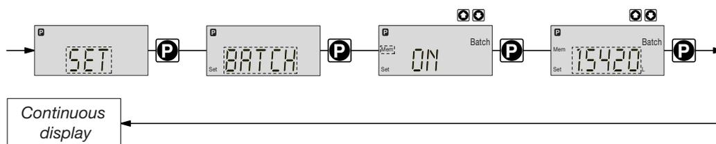
The “batch” operating mode is a variant of the “contact” operating mode (see 7.4.3). You can pre-select a stroke number (no breaks, whole numbers only from 1 to 65535) as well as a feed quantity (batch). To switch between entries for “stroke number” and “feed quantity” press the i key 1x in the corresponding menu option (see also overview “operating/settings diagram”, fold-out page).
