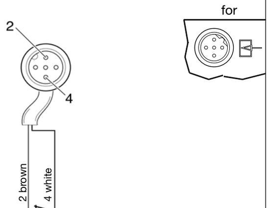
Contact closed -> metering stroke
