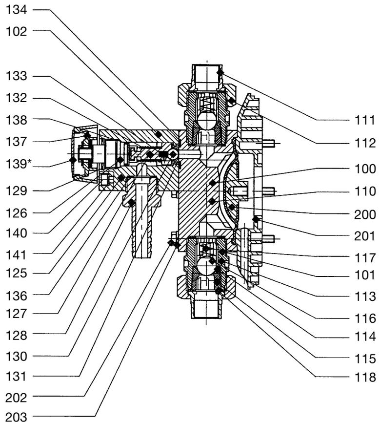
Overflow valve Sigma/ 2 liquid end, 16 bar SST
