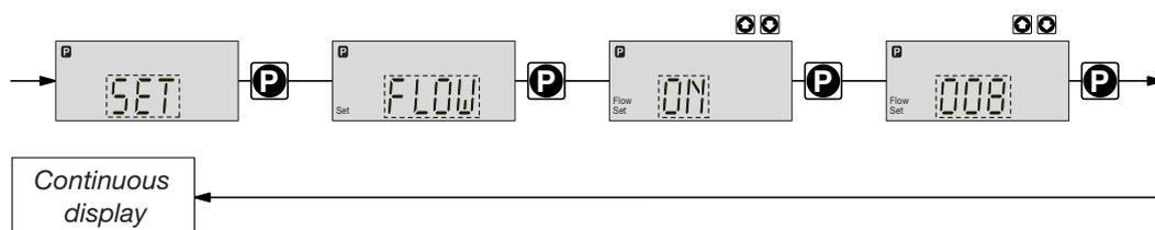
The flow menu only appears when a dosing monitor is connected to the “dosing monitor” terminal. This dosing monitor registers each discharge stroke of the S2Ca at the discharge connector and transmits it back to the S2Ca. If this response transmission is serially omitted for a period set in the FLOW menu (due to failure or below-minimum dosing) the S2Ca stops.
