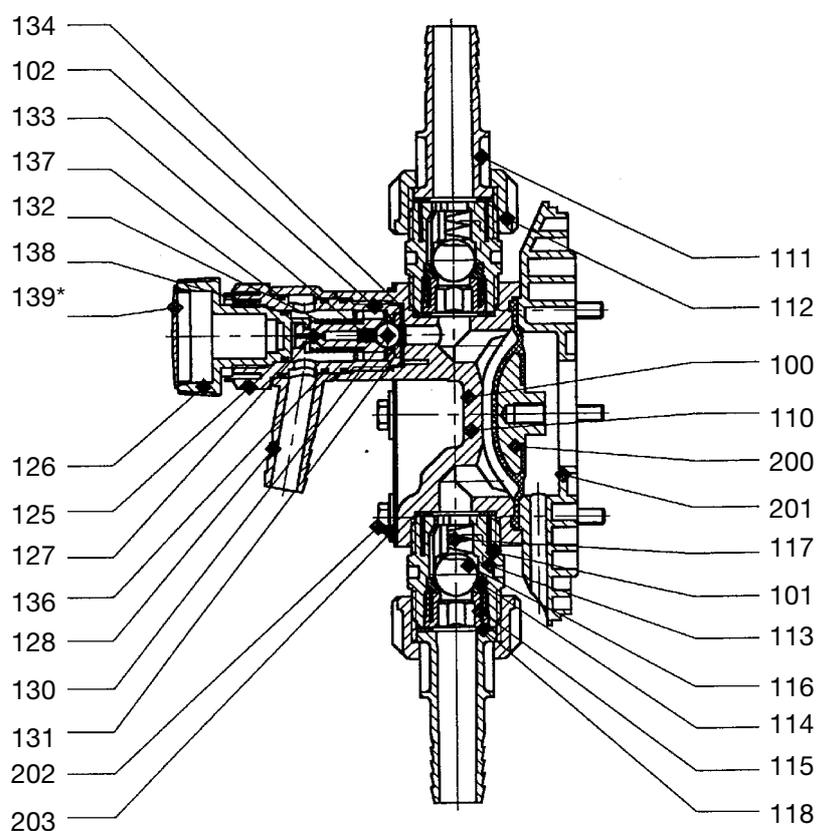
Overflow valve Sigma/ 2 liquid end, 10 bar PVT
