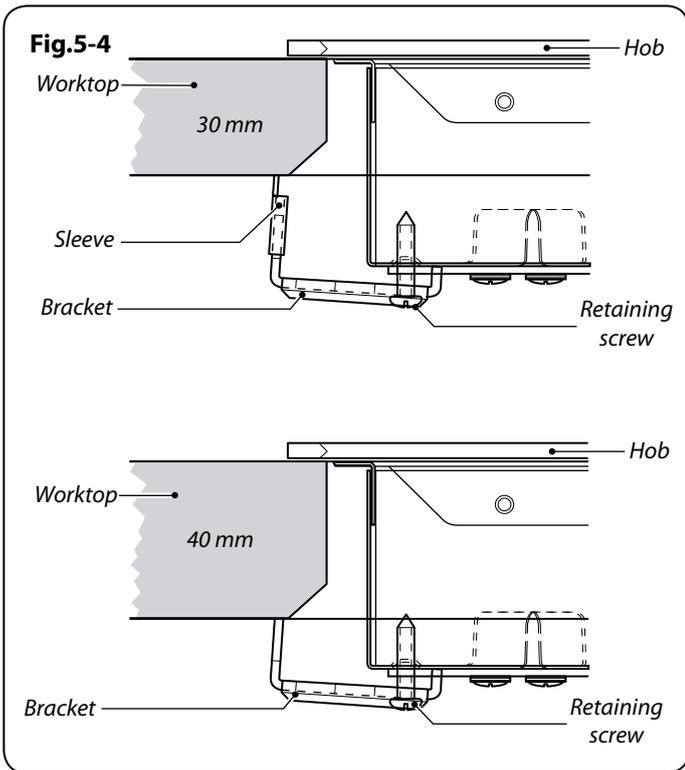
Secure the hob to the worktop using the brackets supplied. The positioning of the bracket (and sleeve) is dependent on the thickness of the worktop as shown in **(Fig.5-4)**.
