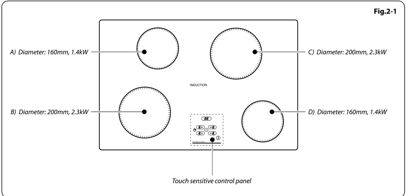
The induction hob comprises of four cooking zones containing induction elements with different ratings and diameters (**Fig.2-1**), each with a pan detector and residual heat indicator. Each zone is controlled via the touch sensitive controls with an audible signal when operated.
