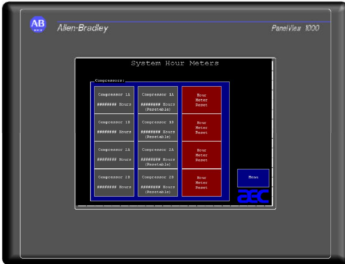
Two hourmeters are kept for each compressor in the system. The first is a lifetime meter. This measures the total time that the compressor has been operational in the lifetime of the chiller. The second is a resettable hourmeter. This hourmeter can be cleared to monitor run time on specific intervals. In order to clear the resettable hourmeter, press the **Hour Meter Reset** button (as prompted on the screen)
