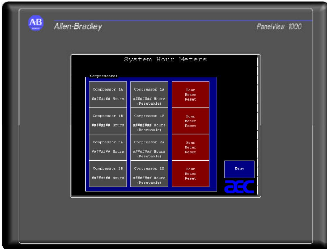
Two hourmeters are kept for each compressor in the system. The first is a lifetime meter. This measures the total time that the pump has been operational in the lifetime of the chiller. The second is a resettable hourmeter. This hourmeter can be cleared to monitor run time on specific intervals. In order to clear the resettable hourmeter, press the appropriate “Hour Meter Reset” button (as prompted on the screen)
