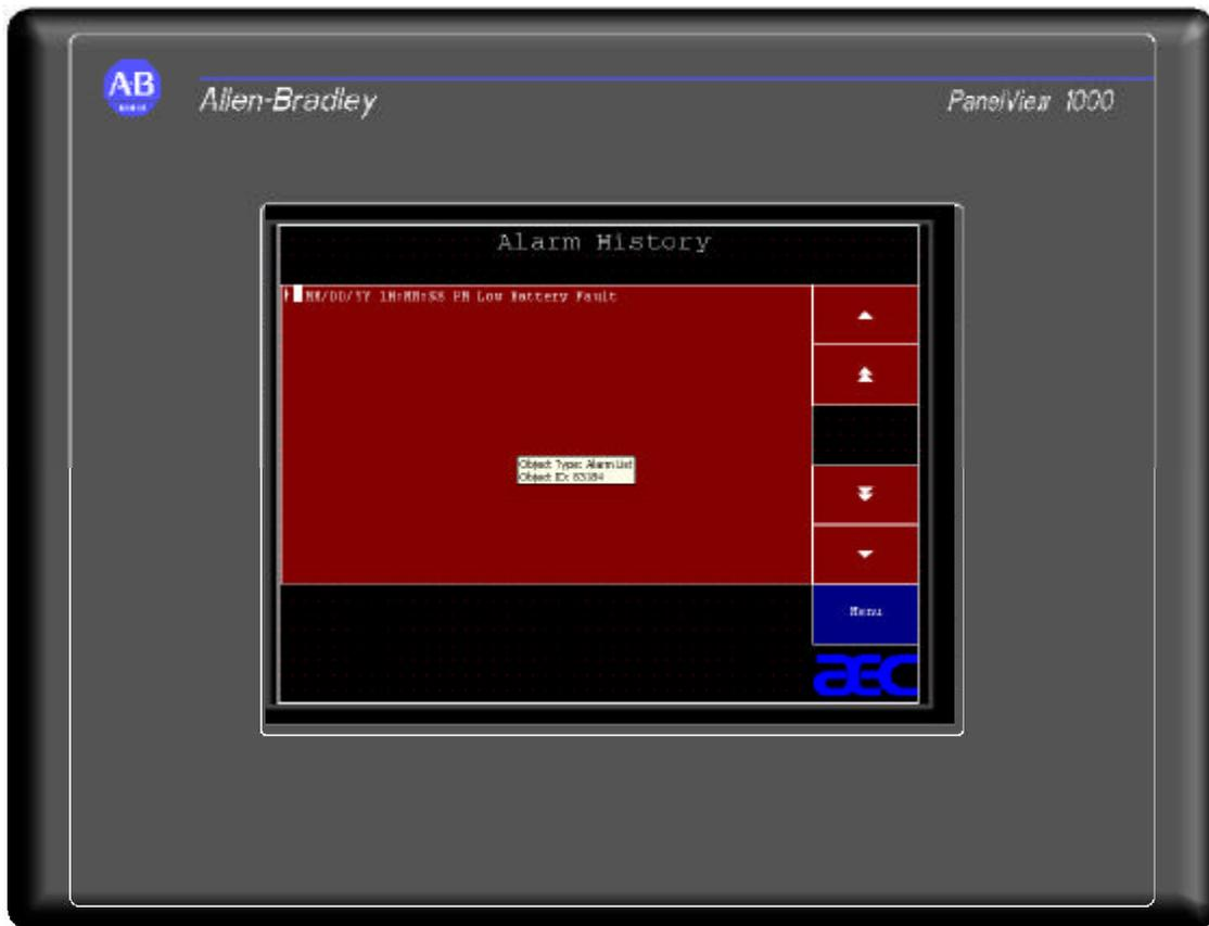
To acknowledge the alarm, press the alarm silence button to clear it. It will then appear in the alarm history screen. Except for High and Low Water Temperature, and Low Refrigerant Pressure, these alarms are considered fatal and maintenance must be preformed in order to allow the chiller to fully run. Should a compressor or
