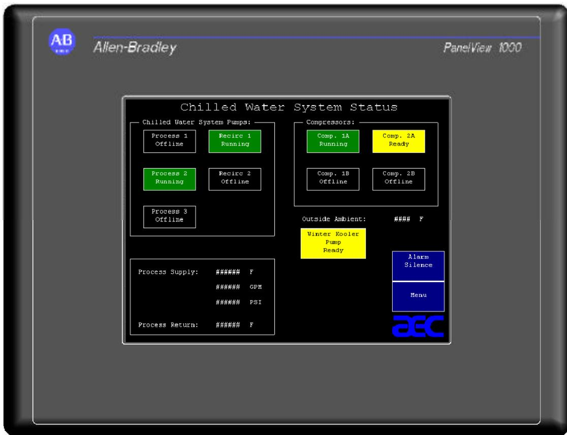
Only pumps that are included in the system will be shown on this screen. Pumps will display one of the following states:
