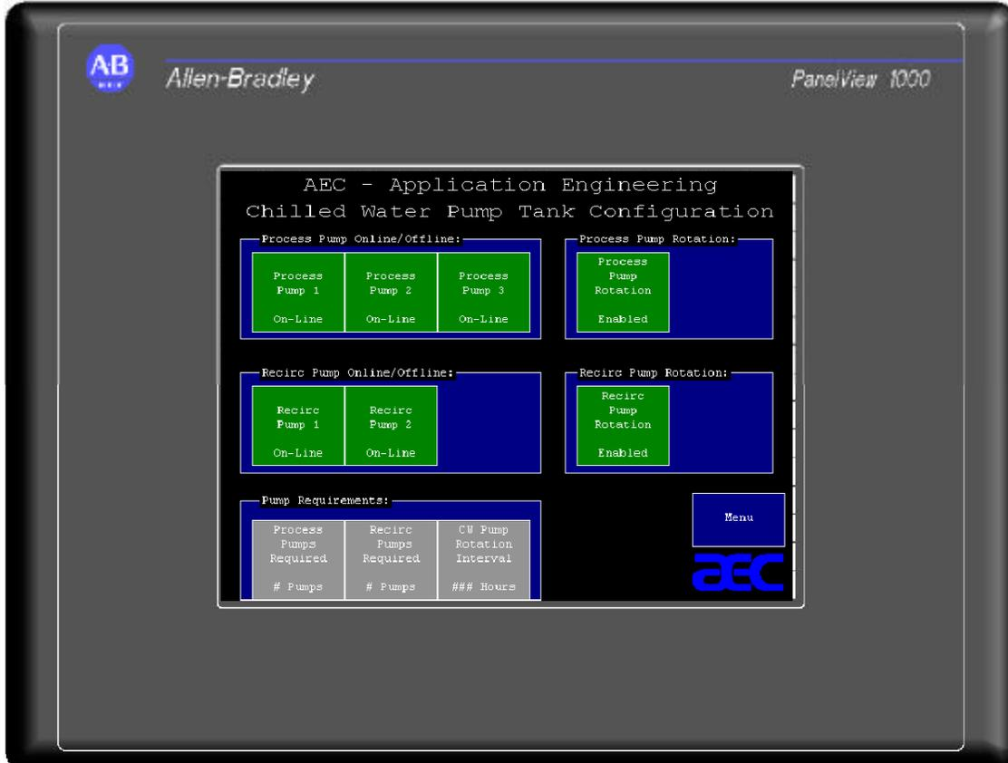
Any pump that is disabled to the OFF-LINE position will not be called to operate. Simply press the button of the desired pump to toggle the state of the pump from the ON-LINE to OFF-LINE state.
