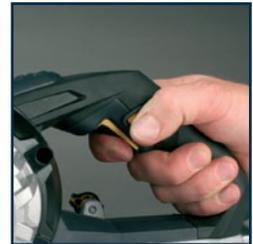
**CAUTION.** Please note that the planer blades continue to spin for some time after switching off the planer. Wait until the motor has completely stopped before setting down the tool to prevent damage to the planer blades or the surface.
