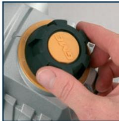
2. The numbers on the ring under the depth adjustment knob indicate the depth of cut. For example when '2.0' is next to the pointer on the front of the planer, the depth of cut is 2mm.
