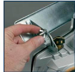
1. Fit the fence guide (14) to the base by screwing the knobs (7) into the fixing points (8).
