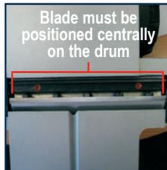
**Note.** Your planing surface will end up rough and uneven unless the blades are set and secured properly.
