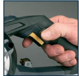
1. Plug in the machine, push in the lock-off button (2) and pull the trigger switch (1).
