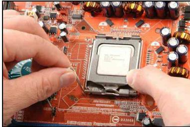
7. Secure the lever with the hook under retention tab.
