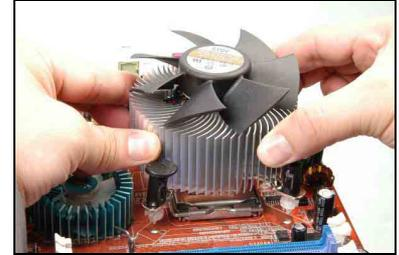
9. Press each of the four fasteners down into the mounting holes. Rotate the fastener clock-wise to lock the heatsink and fan assembly into position.
