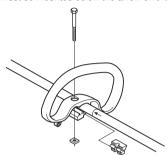
Slide the spacer into the slot in the loop handle. Fit the nut and screw. Tighten.
