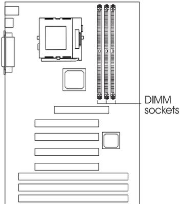
CB60-BX is equipped with three DIMM sockets and CB60-ZX is equipped with two DIMM sockets.
