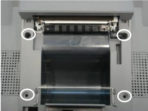
c. Remove the screws (4) to take the module up.
