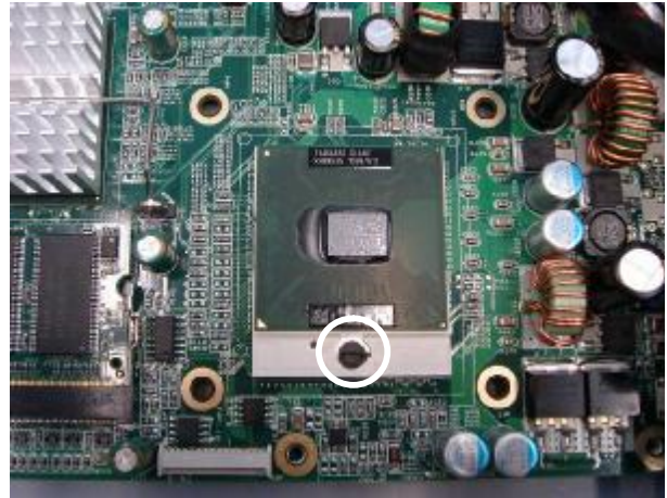
b. Turn the knob 180 degrees to open the key lock to remove the CPU.
