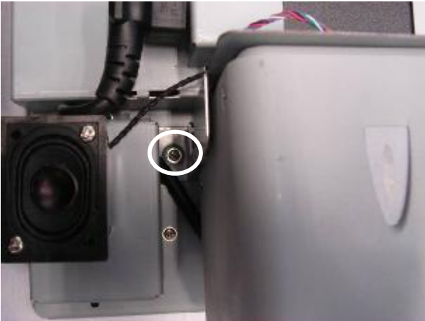
b. Remove the screw (1) to replace the laser scanner.
