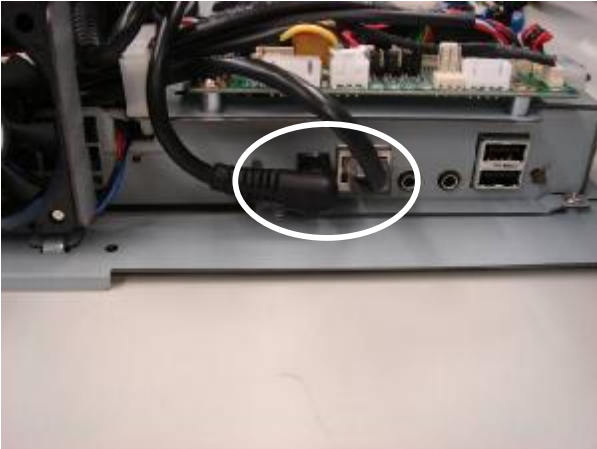
d. Disconnect the cable (2): DC Jack cable (1) and LAN cable (1).
