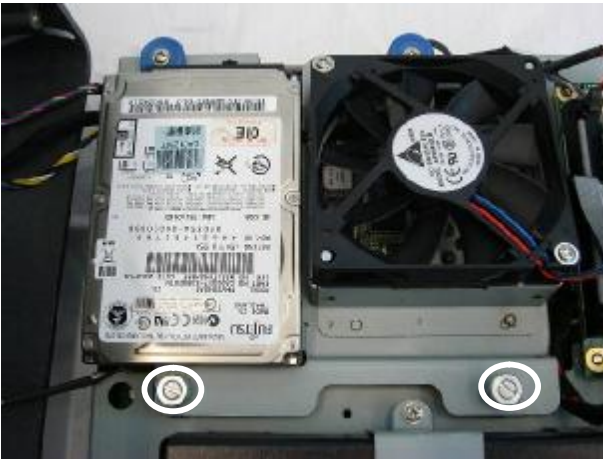
d. Loosen the screws (2) to lift the HDD bracket up.
