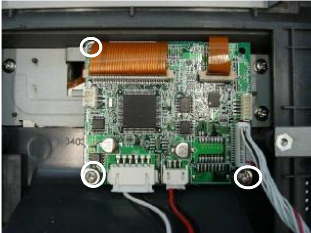
e. Remove the screws (3) to replace the printer control board.
