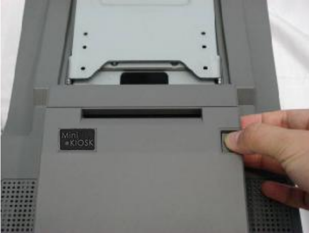
b. Push the button to open the cover.
