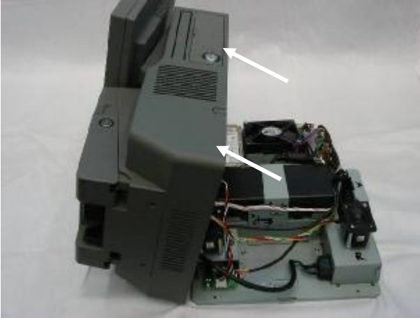
b. Open the main housing to separate it from the base chassis, taking care not to stretch the cables which are still connected. (K811 showed in the picture.)
