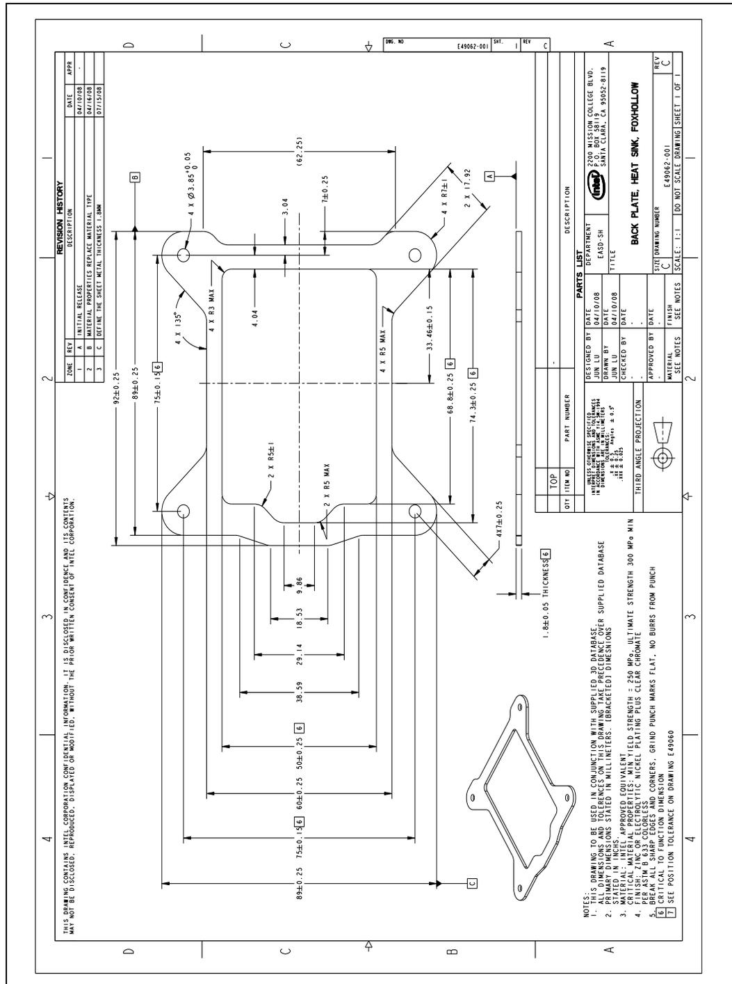
Figure B-15. Heatsink Backplate Insulator
