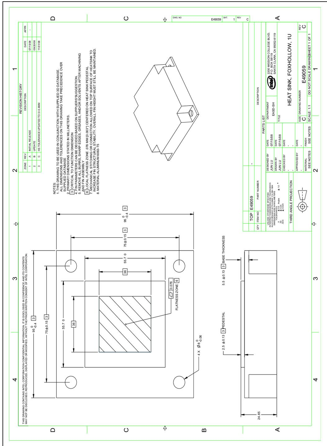
Figure B-7. 1U Reference Heatsink Assembly
