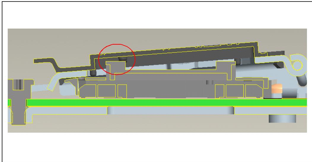
As indicated in [Figure 4-7](#), the pick and place cover cannot remain in place and used in conjunction with the ILM Cover. The ILM Cover is designed to interfere and pop off if the pick and place cover is unintentionally left in place. The ILM cover will also interfere and pop off if the ILM is closed with a processor in place in the socket.
