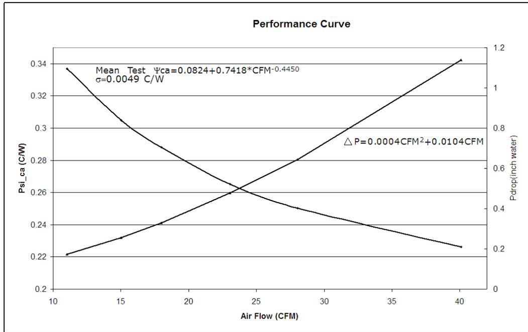
Collaboration thermal solution  $\Psi_{ca}$  (mean+3sigma) is computed to 0.319°C/W at the airflow of 15 CFM. As the Table 9-1 shown when  $T_{LA}$  is 40 °C, equation representing thermal solution of this heatsink is calculated as:
