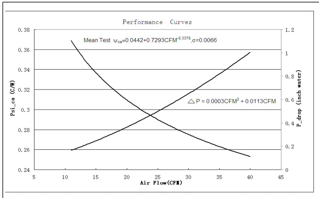
This 1U Reference thermal solution  $\Psi_{ca}(\text{mean}+3\sigma)$  is computed to 0.353°C/W at the airflow of 15.5 CFM, which just meets Intel® Xeon® processor E3-1280 (95W) TTV thermal profile specification when  $T_{LA}$  is 40 °C.
