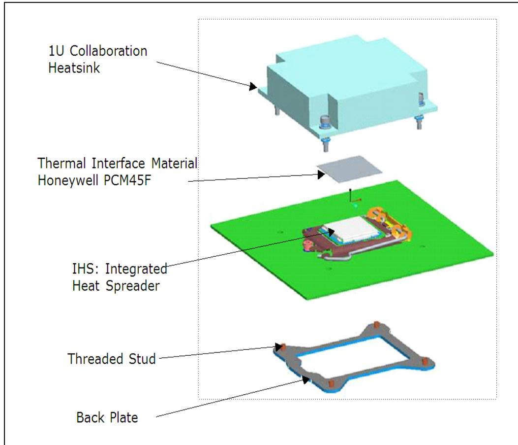
The assembly process for the 1U collaboration heatsink with application of thermal interface material begins with placing back plate in a fixture. The motherboard is aligned with fixture.
