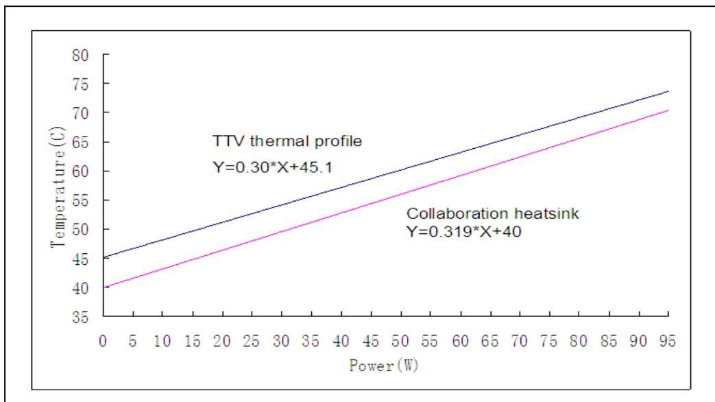
Table 9-2. Comparison between TTV Thermal Profile and Thermal Solution Performance for Intel® Xeon® Processor E3-1280 (95W) (Sheet 1 of 2)
