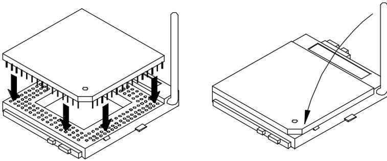
After you have installed the processor into the socket, check if the jumpers for the CPU type and speed are correct.
